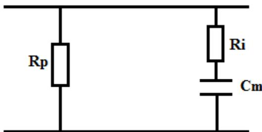
**Figure 1.** Three-element model of blood.  $R_p$  represents plasma resistance,  $R_i$  is cell interior resistance and  $C_m$  is cell membrane capacitance.
