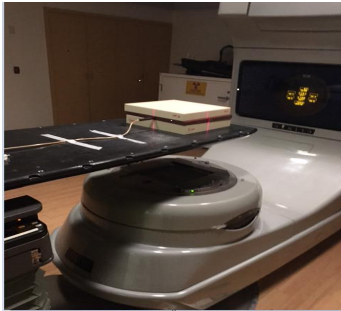
Figure 2a: Setup for the beam attenuation measurement as a function of photon energy and gantry rotation through 10 cm solid water slab
