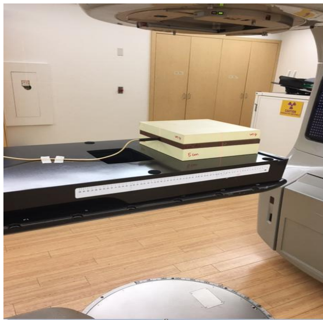
Figure 2b: Setup for the beam attenuation measurement as a function of photon energy and gantry rotation through 10 cm solid water slab and a carbon-fiber belly board
